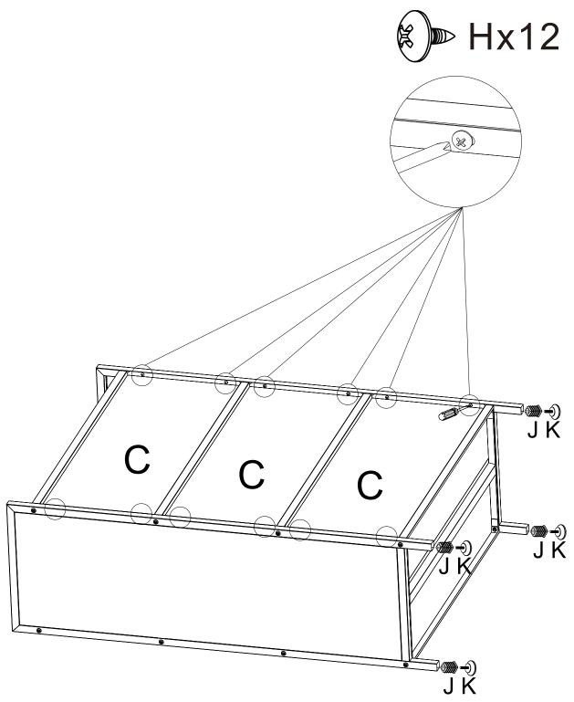
Insert the foot plug J and then twist in the adjustment foot K.
